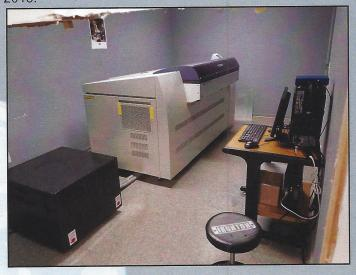
This plate maker makes the plates for all our presses. It took 30 minutes for our old system to make a plate. This new system makes a plate in about 4 minutes with no chemicals. As with all of our equipment, it is a used one but was refurbished and built to last for many years. Praise the name of the Lord for His great blessings!
